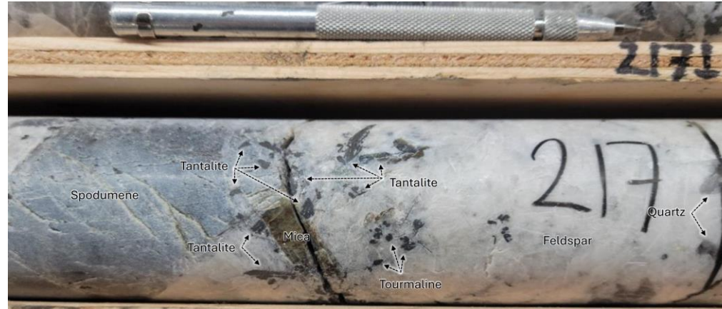
Very coarse-grained tantalite crystals proximal to large spodumene crystal at ~217 m depth in drill hole CV23-109 at the CV5 Pegmatite. Core grades 1,688 ppm Ta 2 O 5 over 0.5 m (216.5 m to 217.0 m) 1
