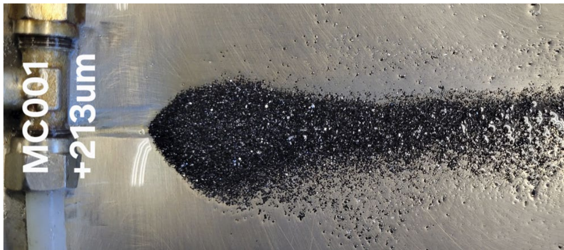
Concentrate from Mozley table testwork from CV5 drill core composite MC001. Tantalum grade and recovery results are not yet known.
