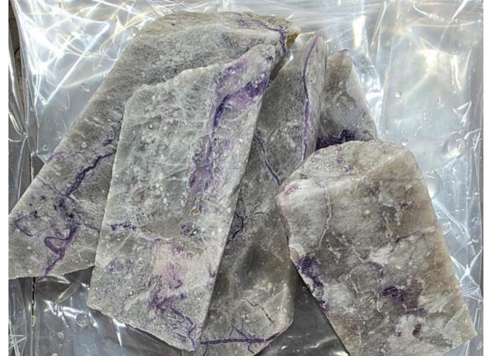
Pollucite core composite (~30% Cs<sub>2</sub>O) from Vega (CV13 Pegmatite). Used as XRT ore sorter training set.
