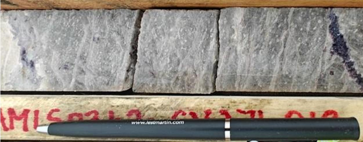
Pollucite mineralization in high-grade caesium drill intersection at ~64.5 m depth in drill hole CV23-271 at the Rigel Zone, CV13 Pegmatite. Interval grades 22.69% Cs<sub>2</sub>O over 1.0 m (64.0 m to 65.0 m)<sup>1</sup>
