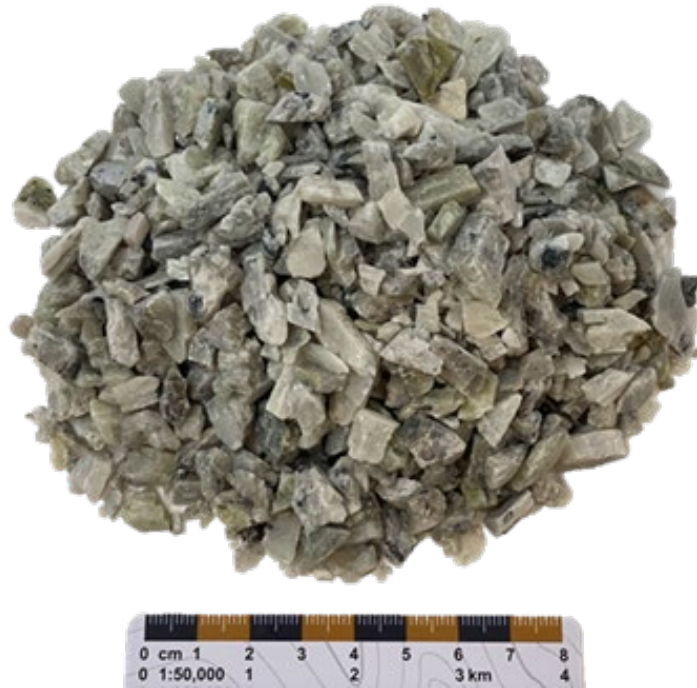
Figure 1.6: Final Concentrate Product Generated from the CV5 Pegmatite via DMS
